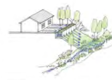
Flow through planter into a bilk. Flows from the underdrain and overflow must be directed in accordance with local requirements.
