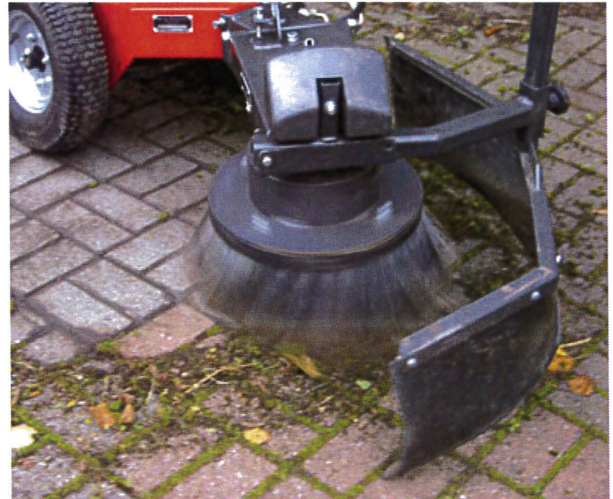
Motor-driven Weed Brush (Kersten WeedBrush®)
