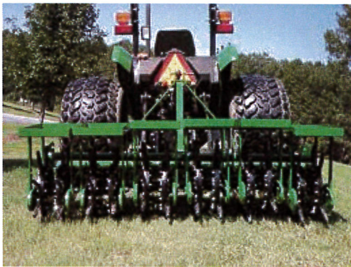
Pull-behind, cam-driven aerator
